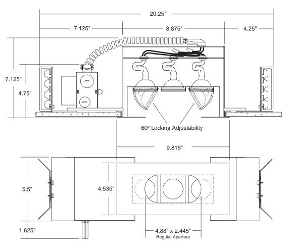
Provided with two (2) 14 gauge steel butterfly type brackets for black iron installations.
